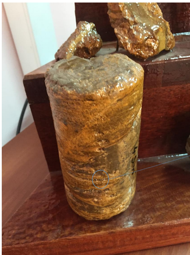
Figure 4: Sediment samples showing effect of grouting
